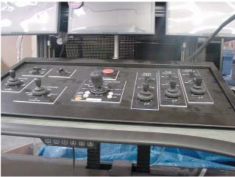
Crane operator’s control panel with six joysticks to be used in the Waste Treatment and Immobilization Plant (WTP) under construction at the U.S. Department of Energy’s Hanford, WA, site by Bechtel. Image courtesy of Washington Group.
